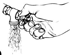
Before attaching water inlet hose, run water through both faucets into a bucket. This will get rid of particles in the water lines that might clog hoses. Mark which is the hot water faucet.
